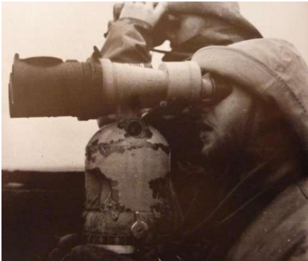
Picture 2; UDF with hoods on UZO mount; the picture was taken in April 1942, on U-373; Picture No 1 and 2 are from book: "Wolfpack U-boats at war 1939-1945", by Philip Kaplan and Jack Currie. 1 The book is in our collection.
