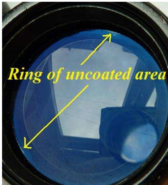
Pict 19; DF 8 x 60H Carl Zeiss Jena with uncoated area; Copyrights pictures Anna Vacani
