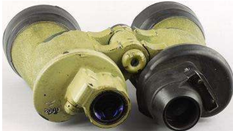
Pict 102; 7 x 50 blc (third model), coated, from Dr Robert Forslund collection; Pictured by Dr R. Forslund; Copyrights Dr Robert Forslund
