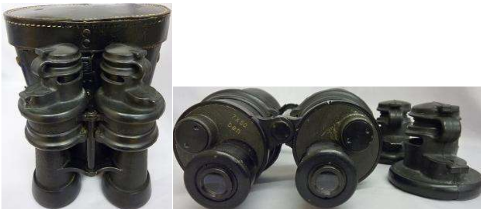
Pict 10; 7 X 50 beh (Leitz) No474230 (late model) in our collection; Copyrights pictures Anna Vacani This model is fitted with desiccator cartridges. The binocular is with Porro II prisms system. This model was built for marine use – on the surface vessels and on U-Boats as well. It is well armored with thick rubber.
