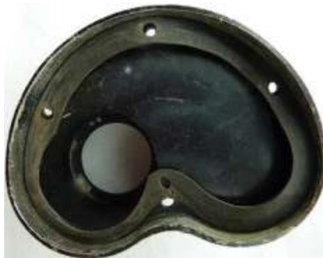
Pict 91; 7 x 50 U-boat - the cover plate with the rubber seal, from our collection; Copyrights of the picture Anna Vacani
