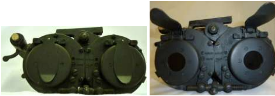
Pict 49; Bausch & Lomb MK 91 Mod 1; the objectives covers and; the eye distance adjustment; copyrights pictures Anna Vacani
