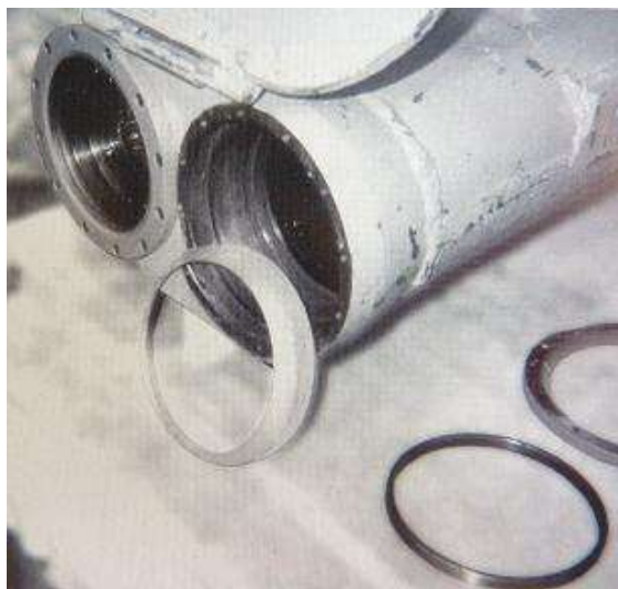
Pict 38; 20 x 120 Japan, the pressure element in front of objective; the picture from Dr Hans Seeger book – 'Militärische Ferngläser und Fernrohre in Heer, Luftwaffe und Marine' ('gray'); page 272; Photograph and description Kevin K. Kuhne
