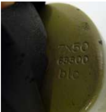
Pict 68; the right plate - under rubber cover engraved "7 x 50 blc" and production number
