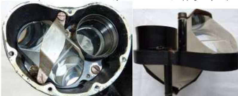
Pict 92; 8 x 60 u-boat prism fitted in the body and prism in the prism shelter ; Copyrights of the picture Anna Vacani
