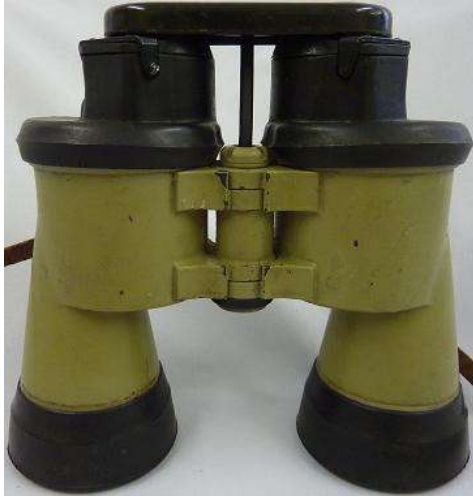
Pict 66; The 7 x 50 U-boat binocular, prod No 63300 (finished with smooth green paint) from our collection; Copyright of the picture Anna Vacani Later version the rubber cord is inserted into the guide on top of the upper hinge (Pict 66).
