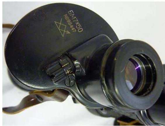
Pict 105; BM 7 x 50 Russian, the binoculars' description on the left plate and the focus adjustment; Copyrights of the picture Anna Vacani
