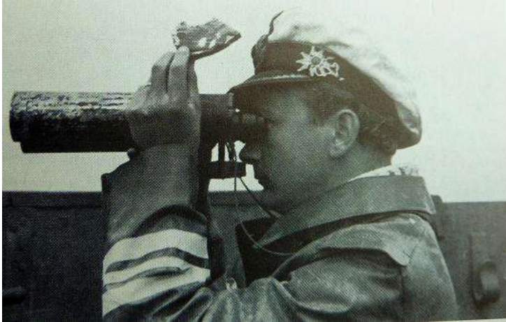
Pict 14; 7 x 50 blc with improvised sunshields; Picture from "U-Boats in the Atlantic; World War 2 Photo Album No 11" by Paul Beaver; in our collection
