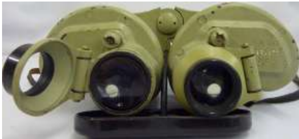
Pict 73; The Bakelite eyecup of the 8 x 60 U-boat binocular, prod No 2111188 from our collection; Copyright of the picture Anna Vacani
