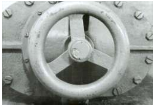
A CLOSER VIEW OF TO REAR WATERTIGHT HATCH WHICH IS CONTROLLED BY A LOCKING WHEEL. THE EYEPIECES CAN BE ADJUSTED FOR EYE SEPARATION. ON THE INSIDE SURFACE OF THIS HATCH IS THE IDENTIFICATION PLATE. IT SHOWS A PRODUCTION DATE OF OCTOBER 1944 WITH THE SERIAL NUMBER 311. ALSO PRESENT IS THE NIKKO LOGO USED BY NIPPON KOGAKU; BOTH BEFORE, DURING AND AFTER THE WAR. R. LINE
