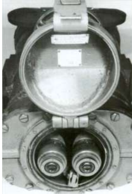
A CLOSER VIEW OF TO REAR WATERTIGHT HATCH WHICH IS CONTROLLED BY A LOCKING WHEEL. THE EYEPIECES CAN BE ADJUSTED FOR EYE SEPARATION. ON THE INSIDE SURFACE OF THIS HATCH IS THE IDENTIFICATION PLATE. IT SHOWS A PRODUCTION DATE OF OCTOBER 1944 WITH THE SERIAL NUMBER 311. ALSO PRESENT IS THE NIKKO LOGO USED BY NIPPON KOGAKU; BOTH BEFORE, DURING AND AFTER THE WAR. R. LINE
