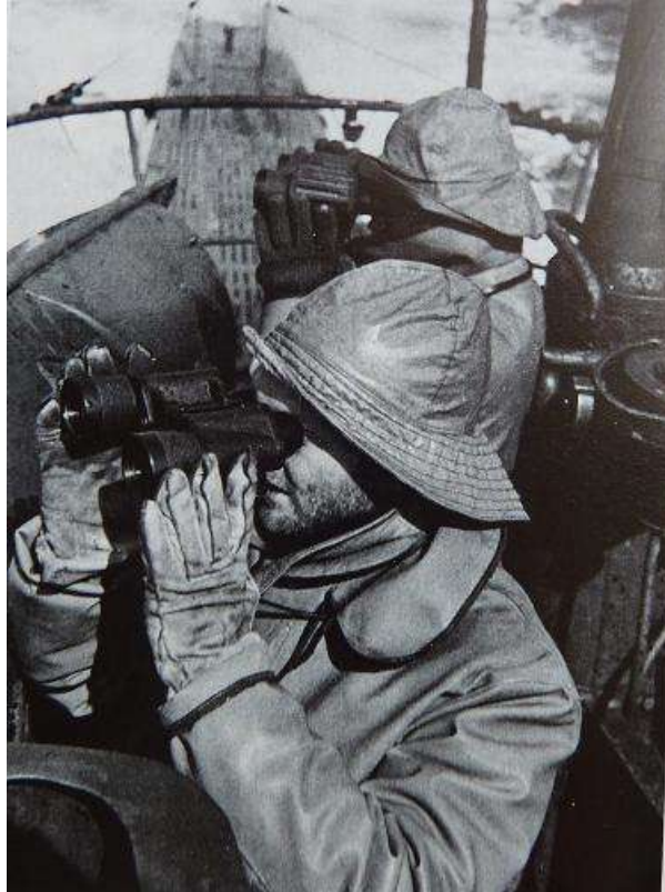
Pict 7; On the U-552; on the conning tower; 7 x 50 Zeiss smooth eyepiece barrel and 7 x 50 Zeiss rubber armored
