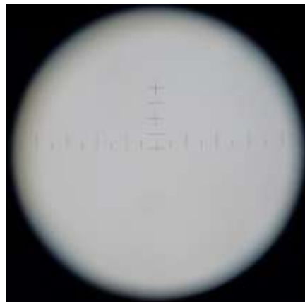
Pict 108; The graticule in the left side Russian 7 x 50 BM model; Copyrights of the picture Anna Vacani
