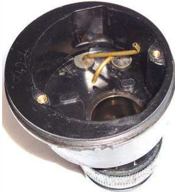
Binocular is internally fitted with selectable green, grey and yellow filters.
