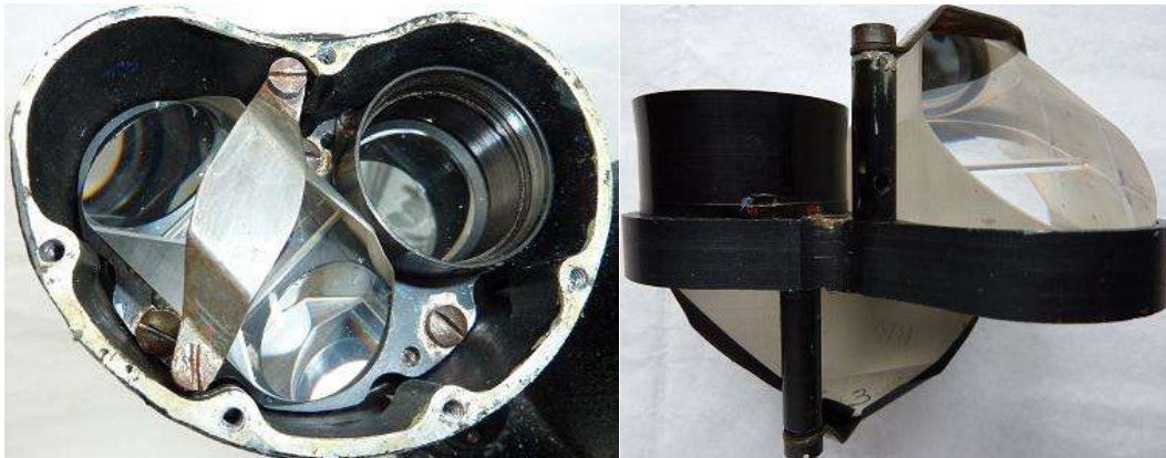
Pict 97; 8 x 60 u-boat prism fitted in the body and prism in the prism shelter ; Copyrights of the picture Anna Vacani
