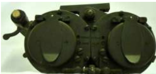
Pict 52; Bausch & Lomb MK 91 Mod 1; the objectives covers and; the eye distance adjustment; copyrights pictures Anna Vacani
