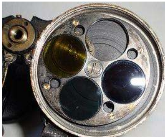
Binocular is internally fitted with selectable green, grey and yellow filters.
