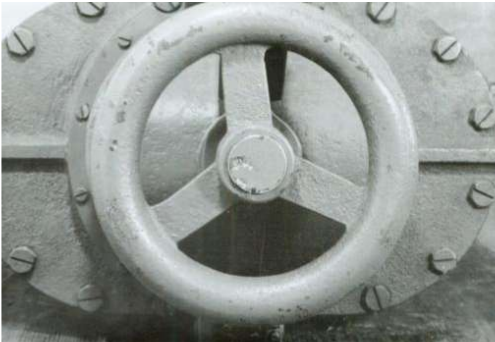
A CLOSER VIEW OF TO REAR WATERTIGHT HATCH WICH IS CONTROLLED BY A LOCKING WHEEL. THE EYEPIECES CAN BE ADJUSTED FOR EYE SEPARATION. ON THE INSIDE SURFACE OF THIS HATCH IS THE IDENTIFICATION PLATE. IT SHOWS A PRODUCTION DATE OF OCTCBER 1944 WITH THE SERIAL NUMBER 311. ALSO PRESENT IS THE NIKKO LOGO USED BY NIPPON KOGAKU; BOTH BEFORE, DURING AND AFTER THE WAR. R. LINE
