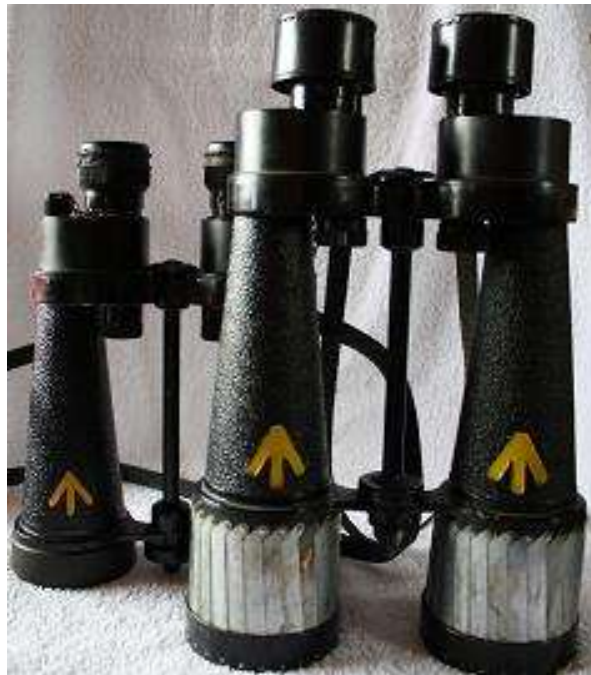
Pict 60; Barr & Stroud CF41 7x50 – with and without desiccator connections, from James Stewart collection, kindly sent for this article; Copyrights pictures James Stewart
