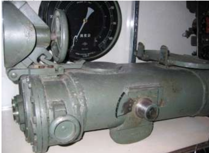
Pict 37; 20x120 type 97 from Richard Lane collection; Picture taken by R. Lane; Copyrights R. Lane Richard Lane says: "The Type 97 binocular prisms are actually larger than a standard Japanese WWII 20x120 (several millimetres on each face)."
