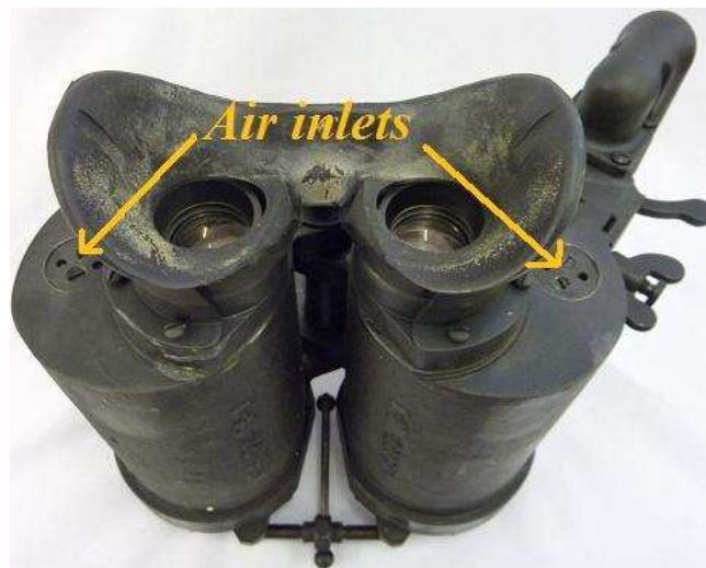
Pict 56; Bausch & Lomb MK 91 Mod 1; the air inlets; copyrights pictures Anna Vacani
