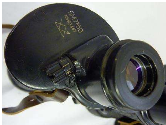
Pict 110; BM 7 x 50 Russian, the binoculars' description on the left plate and the focus adjustment; Copyrights of the picture Anna Vacani
