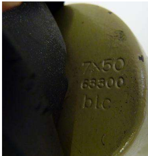
Pict 73; the right plate - under rubber cover engraved "7 x 50 blc" and production number
