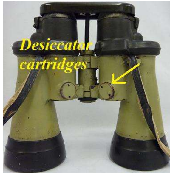
Pict 72; The 7 x 50 U-boat binocular, prod No 56718 from our collection; Copyright of the picture Anna Vacani
