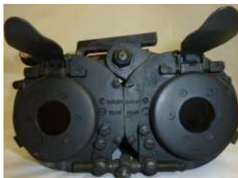
Pict 52; Bausch & Lomb MK 91 Mod 1; the objectives covers and; the eye distance adjustment; copyrights pictures Anna Vacani
