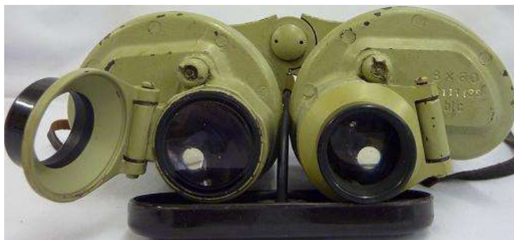
Pict 78; The Bakelite eyecup of the 8 x 60 U-boat binocular, prod No 211188 from our collection; Copyright of the picture Anna Vacani
