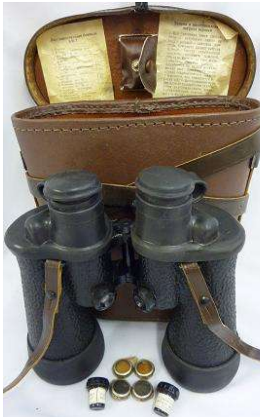
Pict 112; BM 7 x 50 Russian submarine binocular with the original case and accessories; Copyrights of the picture Anna Vacani
