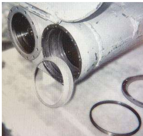
Pict 38; 20 x 120 Japan, the pressure element in front of objective; the picture from Dr Hans Seeger book - Hans T. Seeger - Militrische Fernglser und Fernrohre in Heer, Luftwaffe und Marine; page 272; Photograph and description Kevin K. Kuhne
