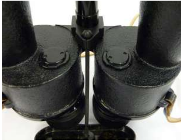
Pict 23; 8 x 60blc, production No 2084791; with desiccator cartridges; Copyrights pictures Anna Vacani
