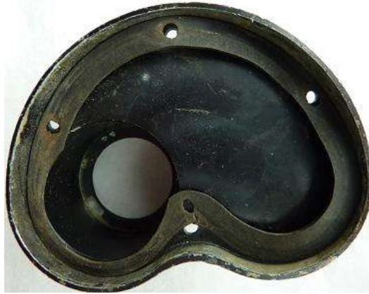
Pict 96; 7 x 50 U-boat - the cover plate with the rubber seal, from our collection; Copyrights of the picture Anna Vacani
