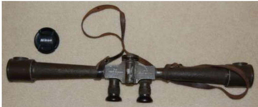
FOS 10x Scissor binocular produced in 1910<sup>7</sup>
