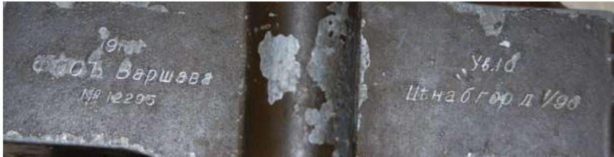
*The description on the scissor binocular: left side – 1910y, FOS Warsaw №12295; right side – magnification 10, graduations of the reticule plate 1/90*
