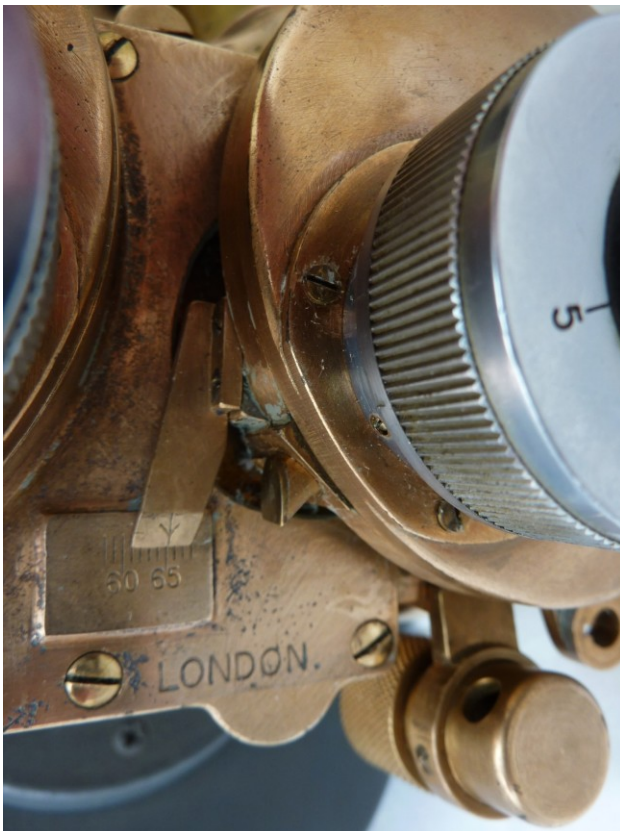
Pict 6; 8 &12, 5 revolver; London V-A. Ltd; eye width adjustment; ©Anna Vacani
