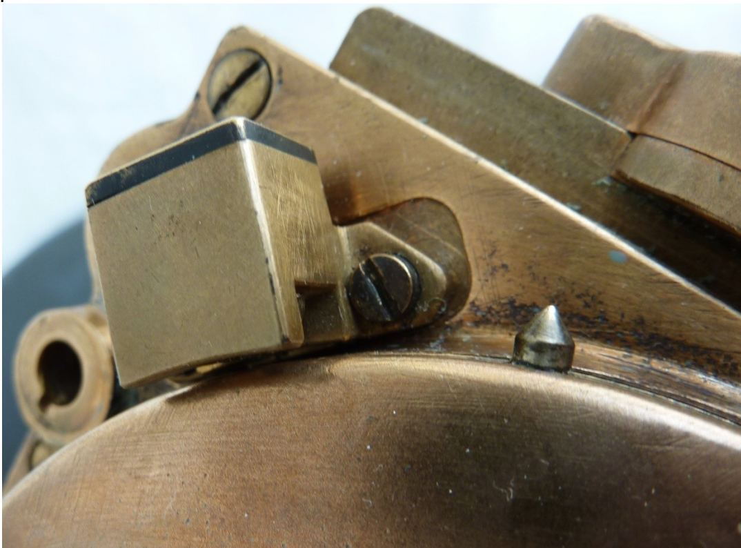
Pict 8; 8 &12, 5 revolver; London V-A. Ltd; stopper for rotation mechanism; ©Anna Vacani
