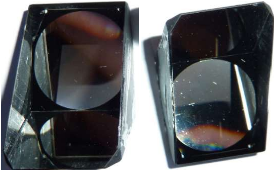
7 x 42 Avimo monocular prototype from our collection – the prism system; Copyrights Anna Vacani
