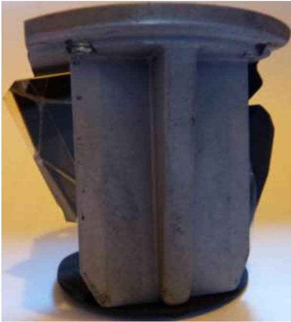
7 x 42 Avimo monocular prototype from our collection – the prisms; Copyrights Anna Vacani
