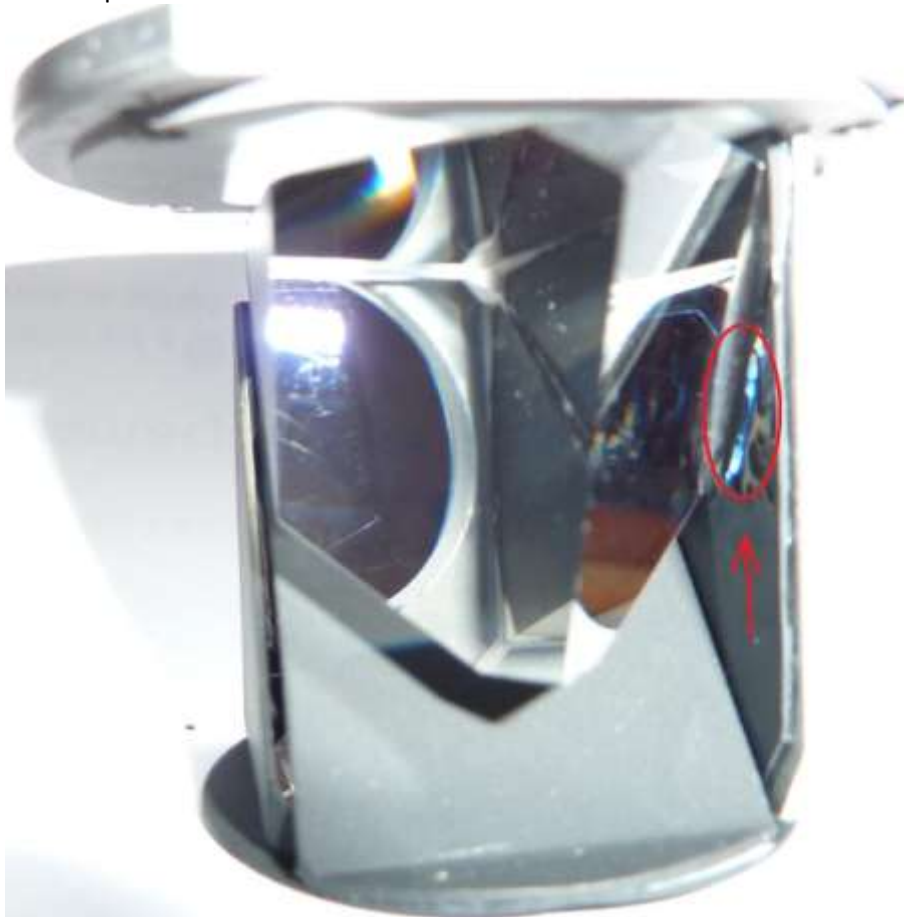
7 x 42 Avimo monocular prototype from our collection – the prism system; Copyrights Anna Vacani
