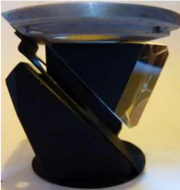
7 x 42 Avimo monocular prototype from our collection – the prisms; Copyrights Anna Vacani
