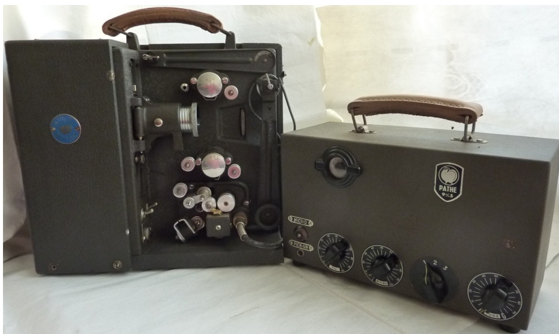
Pict 4b; Pathe Marignan 9,5mm projector with amplifier connected to magnetic head, in our collection; ©Anna Vacani
