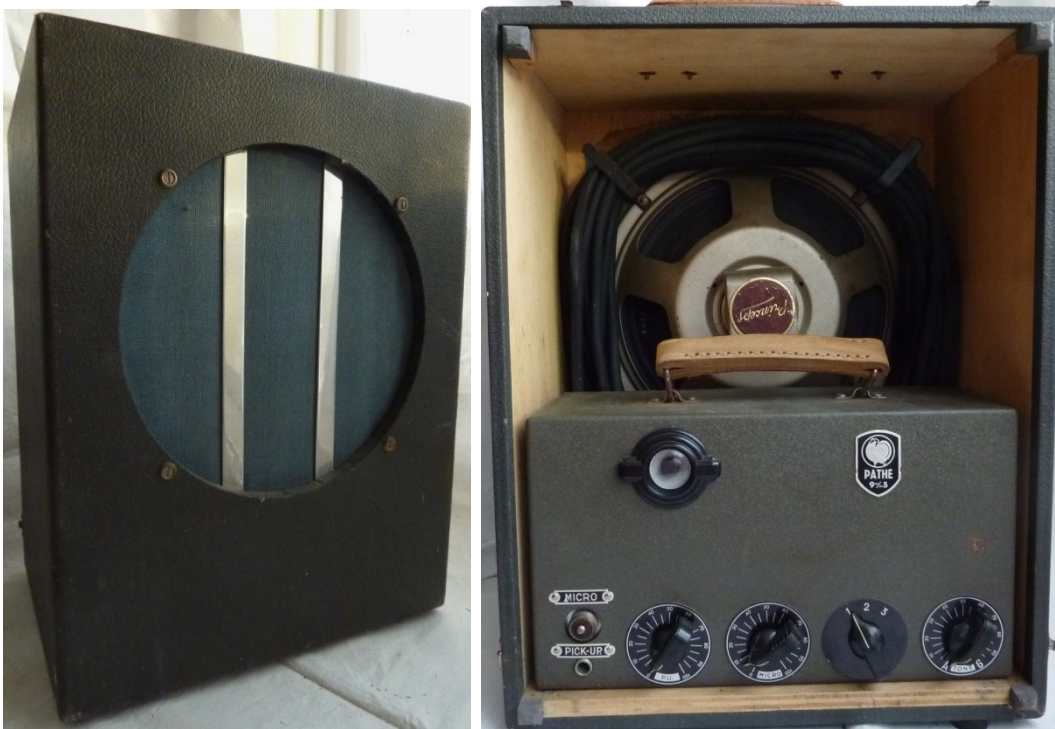
Pict 4c; Amplifier for Pathe Marignan 9,5mm projector, in our collection; ©Anna Vacani
