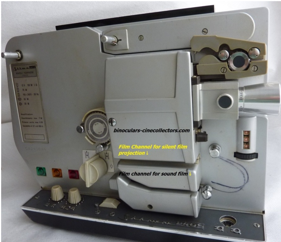
Pict 24; the Silma240S projector- film channels and film counter; ©Anna Vacani
