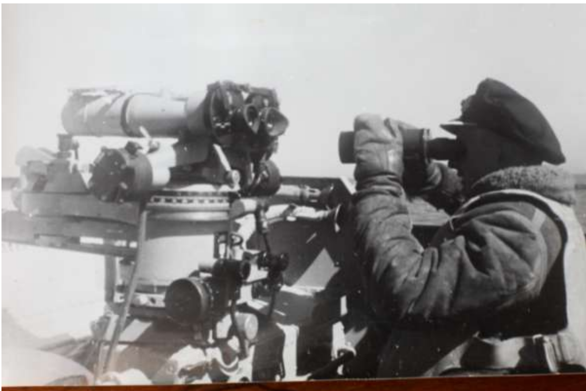
7 x 50 H, on a torpedo director - The picture from Dr Stephen Rohan collection
