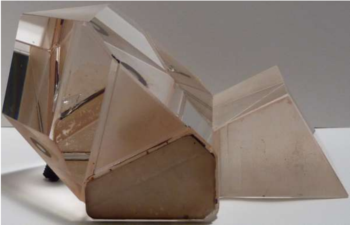
The pictures of the original prism from a damaged binocular
